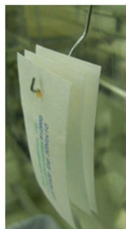
Figure 1. Examples of proper BI configurations when using the hole in the envelope to hang the BI
