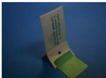
Figure 2. Examples of proper BI configurations when using adhesive tape to position the BI
