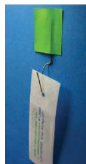
Figure 1. Examples of proper BI configurations when using the hole in the envelope to hang the BI
