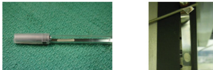
Figure 6. Examples of ribbon BIs in dead leg (left) and hanging on an isolator fixture (right)
