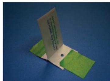
Figure 2. Examples of proper BI configurations when using adhesive tape to position the BI
