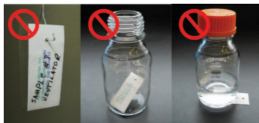
Figure 4. Examples of IMPROPER BI use: writing on the face of the package and placing BI into or underneath a container.
