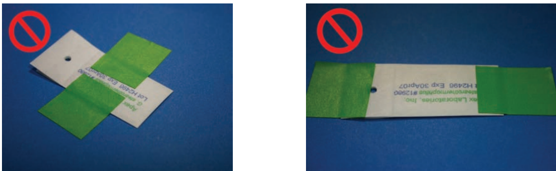
Figure 3. Examples of IMPROPER BI configurations when using adhesive tape
