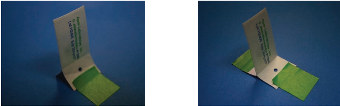
Figure 2. Examples of proper BI configurations when using adhesive tape to position the BI
