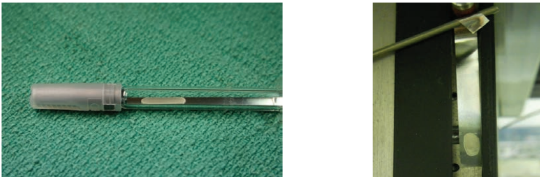
Figure 6. Examples of ribbon BIs in dead leg (left photograph) and hanging on isolator fixture (right photograph)
